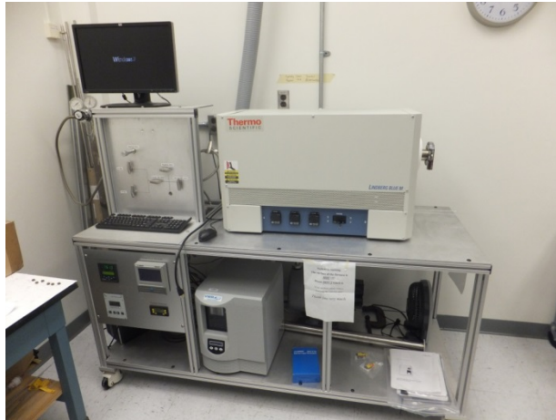
Fig. 116. Hydrogen charging apparatus.
