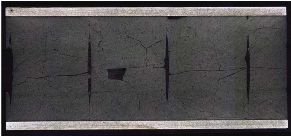
Figure 2. Image of one-inch HBR rod segment from a hot-cell testing sample.
