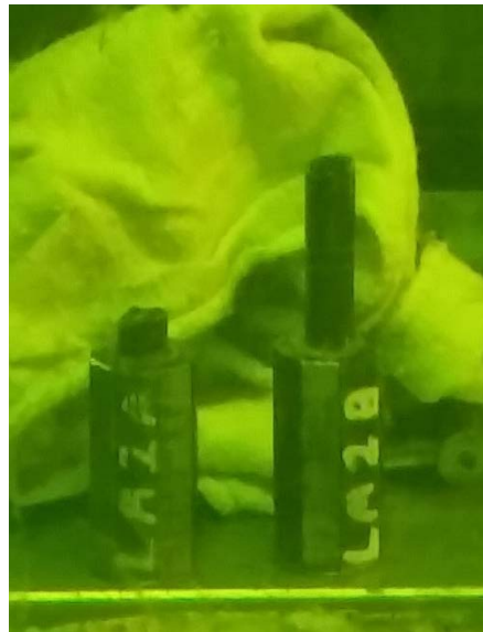
Fig. 10. Fracture segments for LMK02/575D-A; N_f = 1.71 \times 10^5 cycles at \pm 12.70 N·m, 5 Hz.
