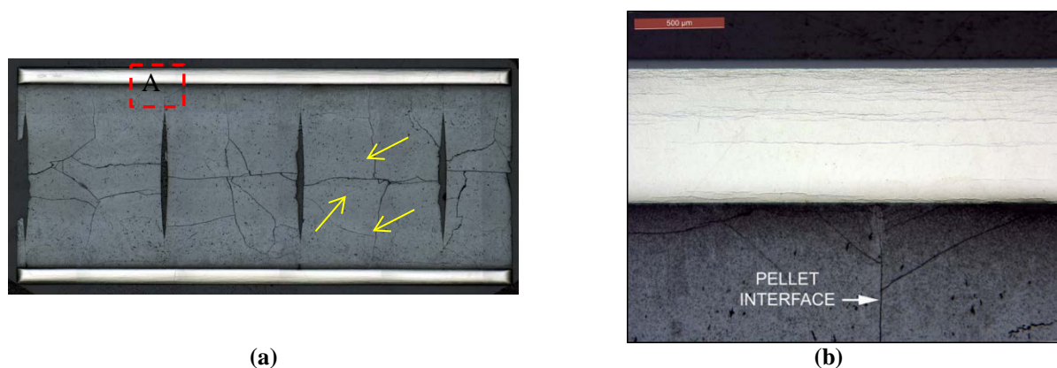
Figure 29. Optical images of untested segment 605D for (a) overall axial cross section and (b) enlarged area A.
