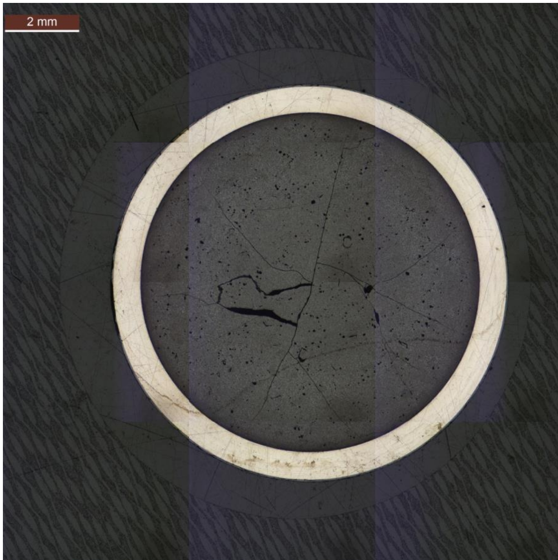
Fig. 115. High-burnup HBR fuel morphology for Sample 607D4A.
