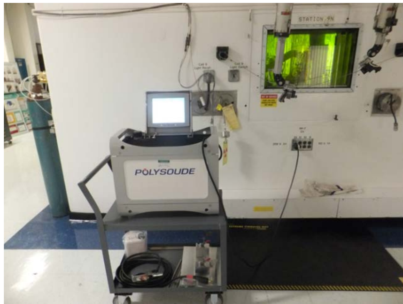
Fig. 118. Astro Arc Polysoude tubing welder.
