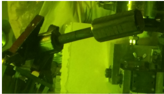
Fig. 13. Fracture segments for LMK03/575B-A N_f = 4.92 \times 10^5 cycles at \pm 10.16 N·m, 5 Hz.
