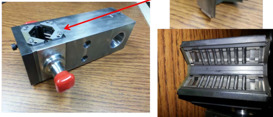
Figure 3. Assembled grip (left) and two views (right) of detached grip body.
