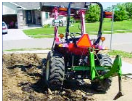
Utilize One-Call to locate all utilities prior to performing deep tillage.
