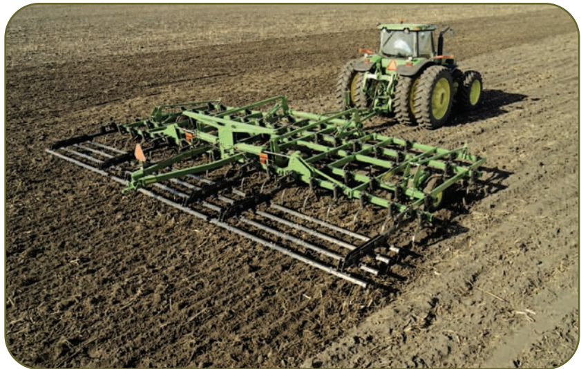
FIELD CULTIVATOR—WITH COILED TINE HARROW
