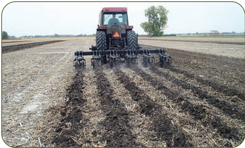
STRIP-TILL AND ZONE-TILL PLANTING SYSTEM
