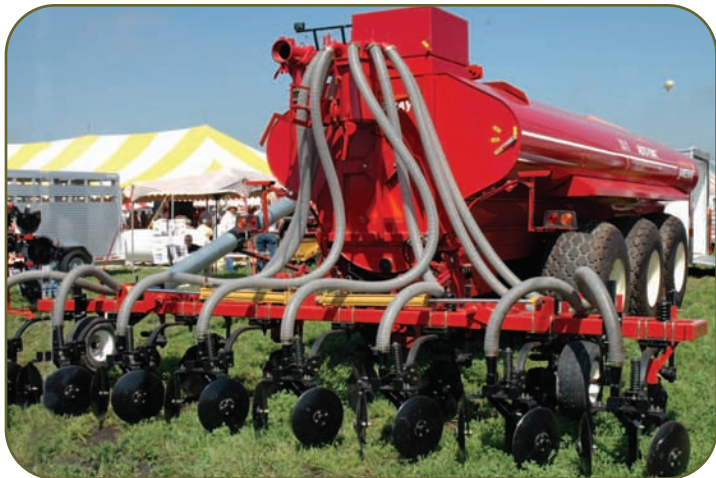
TANK TYPE LIQUID MANURE INJECTOR WITH HIGH DISTURBANCE
