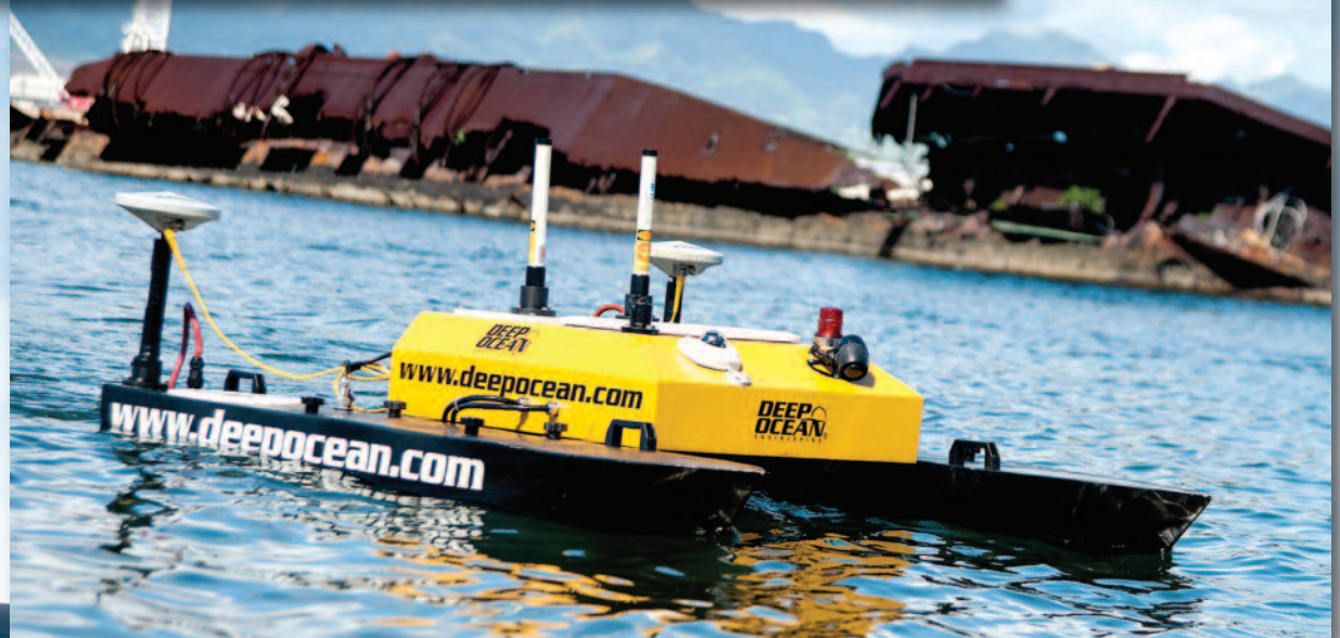
(Right) An unmanned surface vessel from Deep Ocean Engineering conducts multi-beam sonar surveying Oct. 23 at the USS Utah Memorial.
