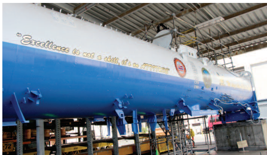
Employees from Pearl Harbor Naval Shipyards, code 740 lifting and handling department, refurbished a former advanced SEAL (sea, air, land) delivery system into a hands-on trainer for all waterfront workers.
