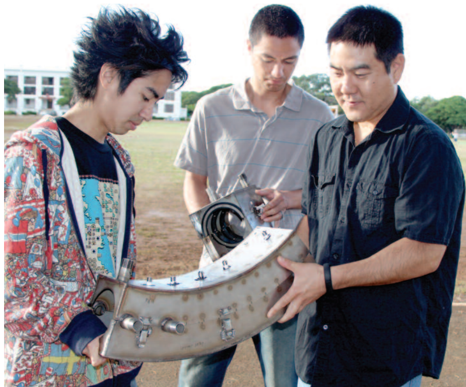
(Left to right) Code 2370's mechanical engineers, Ryan Naka, Noeau Camarillo and Randall Imaoka, put together their innovative freeze seal jacket chamber that uses vacuum techniques to isolate and freeze repair pipes on submarines.
