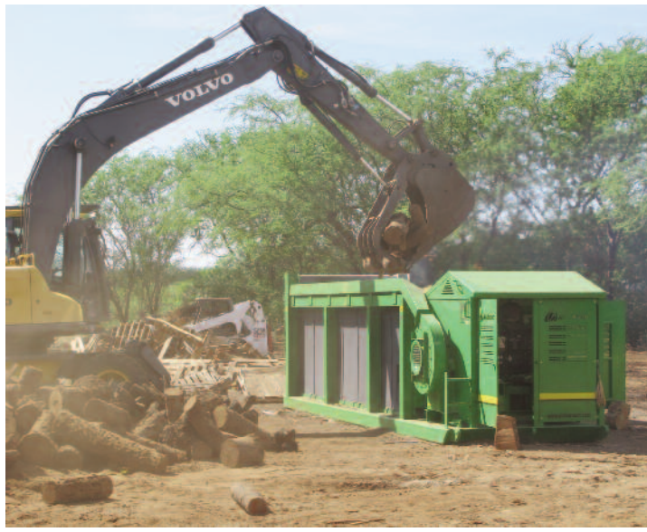
An air curtain burner is loaded with palm logs for incineration. Rotting palm trees can become material for coconut rhinoceros beetle nests.
