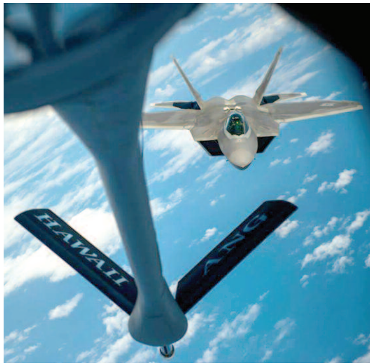
U.S. Air Force photo by Staff Sgt. James Richardson A U.S. Air Force KC-135 Stratotanker from the 96th Air Refueling Wing at joint base refuels a F-22A Raptor from the 199th Fighter Wing during the Rim of the Pacific exercise July 18 over Hawaii.
