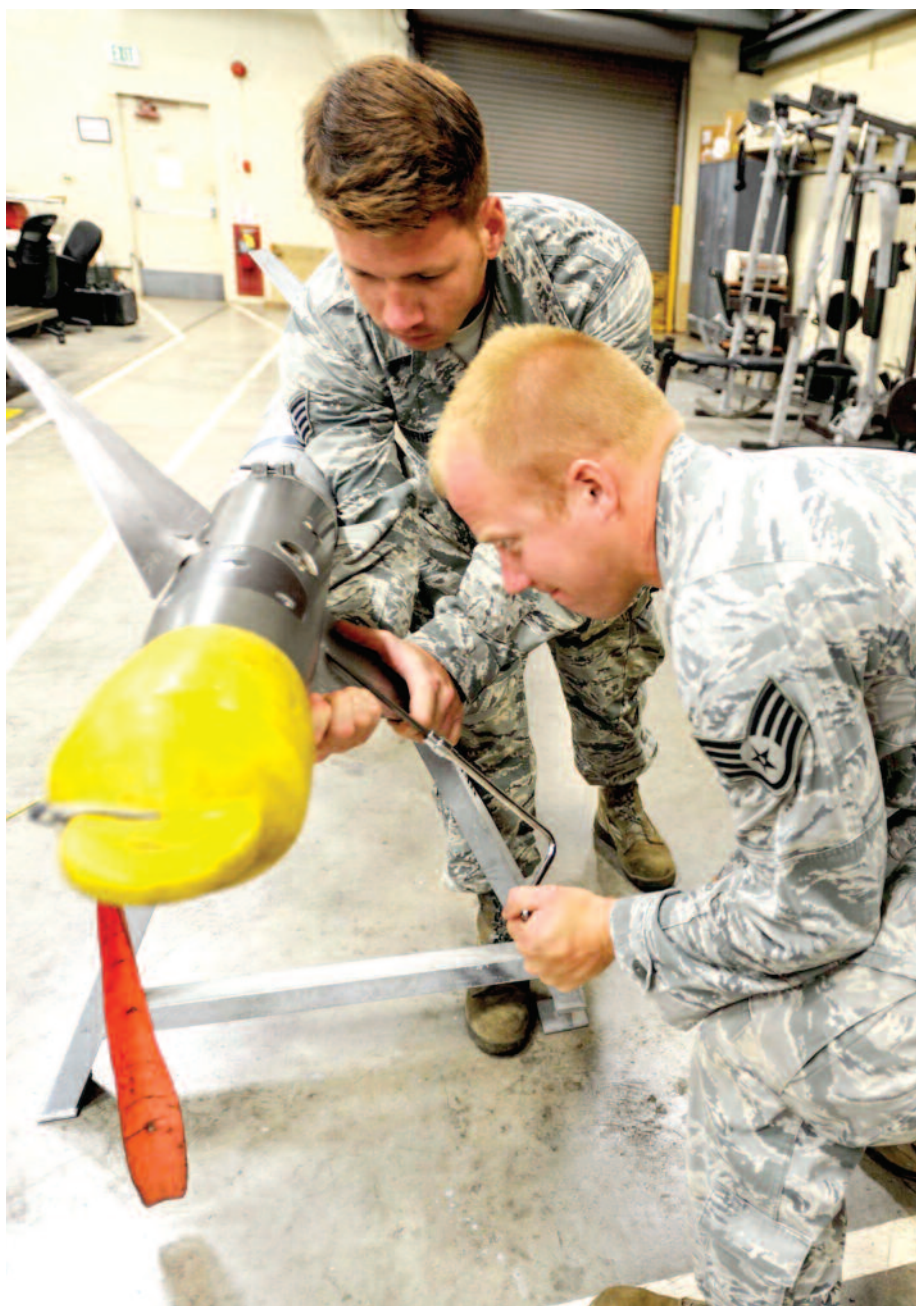
Staff Sgt. Travis Briese, 391st Fighter Squadron (FS) Munitions Flight equipment maintainer, holds a Captive Air Training Missile 9-M fin in place as Staff Sgt. Paul Rinehart, 391st FS Munitions Flight munitions inspector, uses a speed wrench to remove the fin from the guidance section of the missile head July 17.
