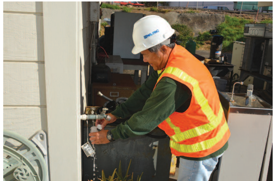
A water distribution system operator from Naval Facilities Engineering Command Hawaii's utilities water production section takes a sample of drinking water from building X29 on the command's main compound on June 11 at Joint Base Pearl Harbor-Hickam.
