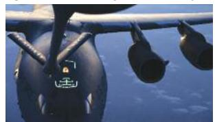
(Above): A C-17 Globemaster III is guided into position behind the boom of a KC-135 Stratotanker in order to receive fuel during an in-air refueling training mission near Joint Base Pearl Harbor-Hickam on March 20.
