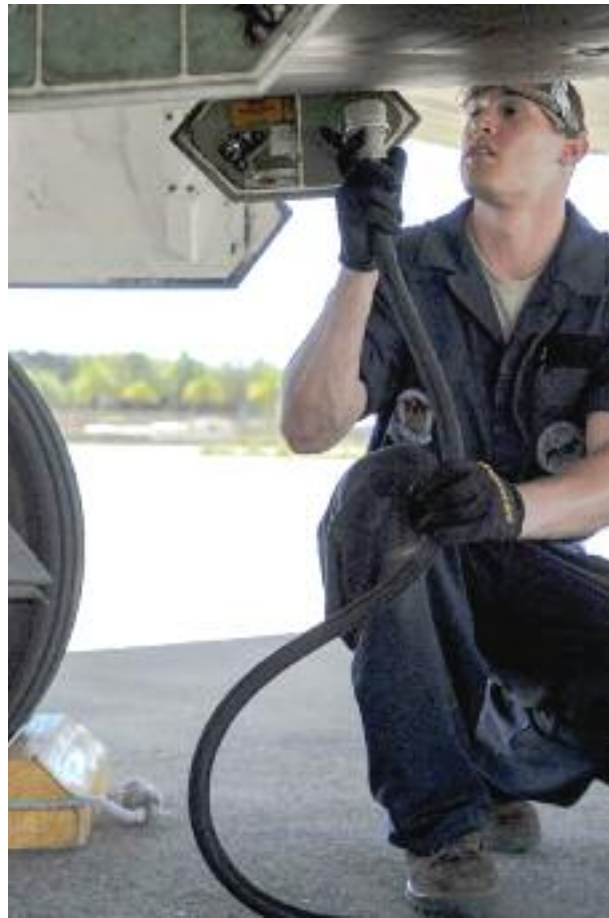
Senior Airman Trey MacLaughlin, a 525th Aircraft Maintenance Unit crew chief, services the oil on an F-22 Raptor engine during a through flight inspection on the flightline at Joint Base Pearl Harbor-Hickam on March 11.
