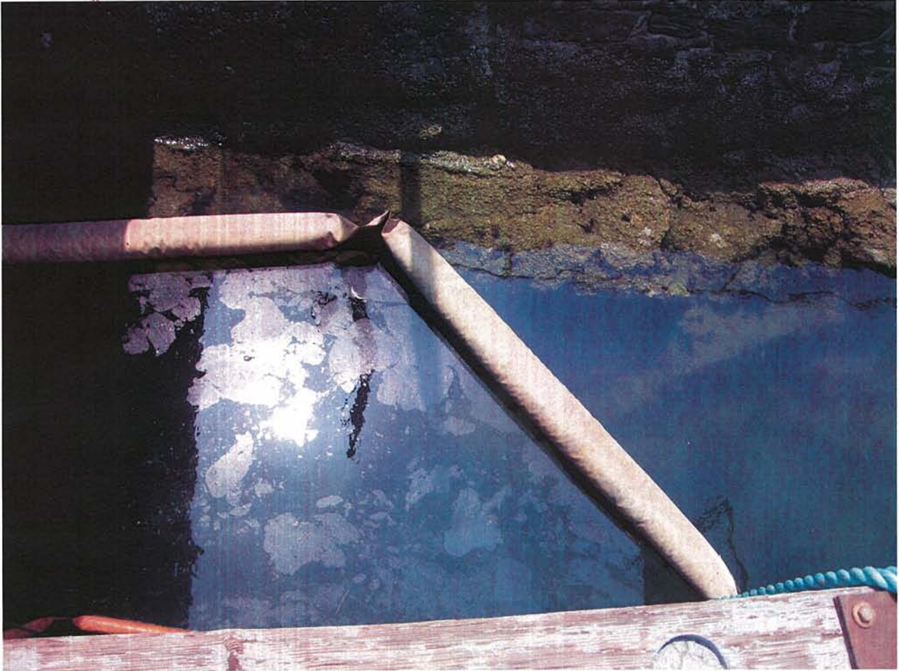
Photo 17: An oil sheen inside the containment boom behind (and below) the fuel dock.
