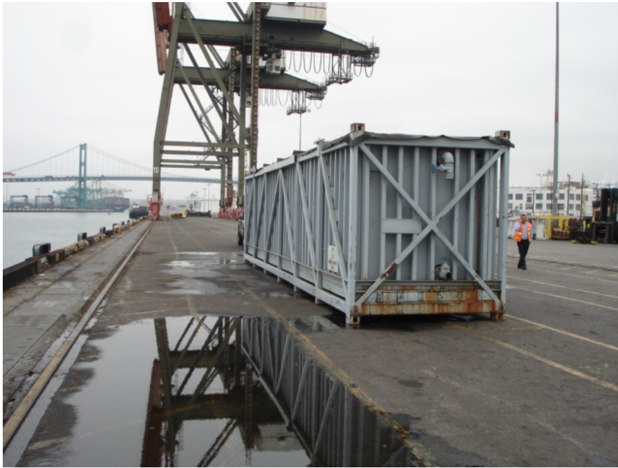
Photo 10: Leaking container used for crane load test
