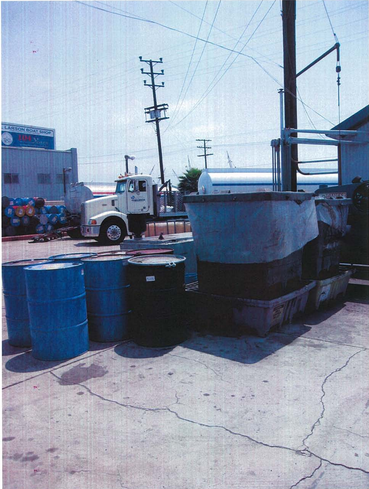
Photo 5: Oil storage area, this area drains off-site storm drains that lead to the Los Angeles Harbor.
