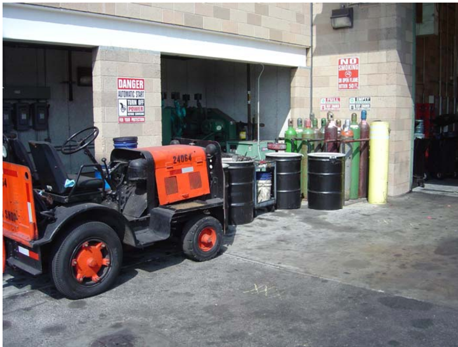
Photo 4: Oil filter drums located outdoors were not on spill pallets.
