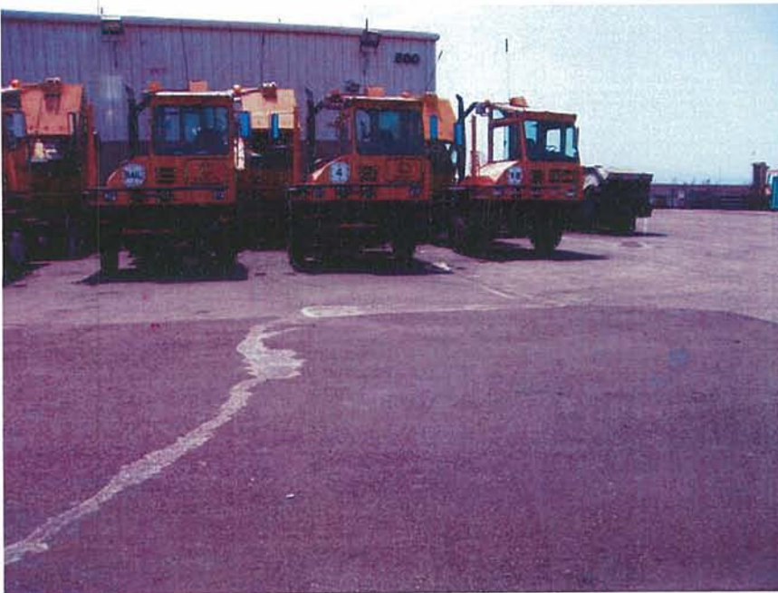
Photo 4 - Flow path of battery acid release to drain inlet.
