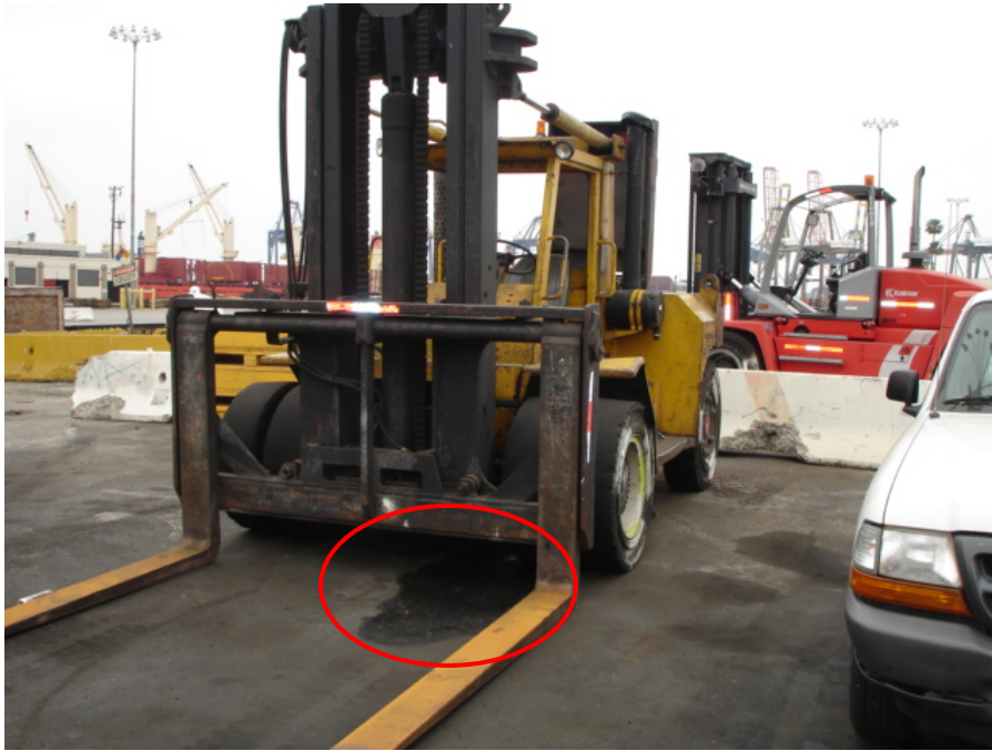
Photo 6: Exposed oil leak adjacent to maintenance shop.
