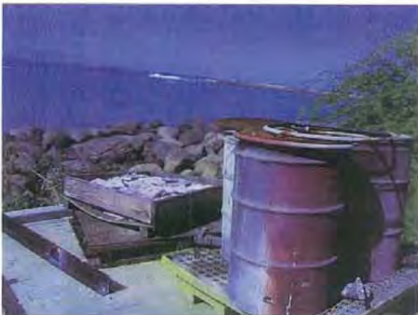
Photo 21: A wooden box of old zinc anodes were observed stored in the area behind the metal working building, exposed to potential rain fall and in the direct drainage area for a nearby storm water discharge location.
