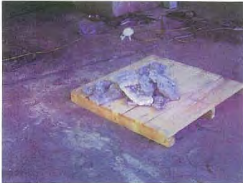
Photo 61: Zinc anodes were observed stored on the dry dock, uncovered and exposed to potential rain fall.
