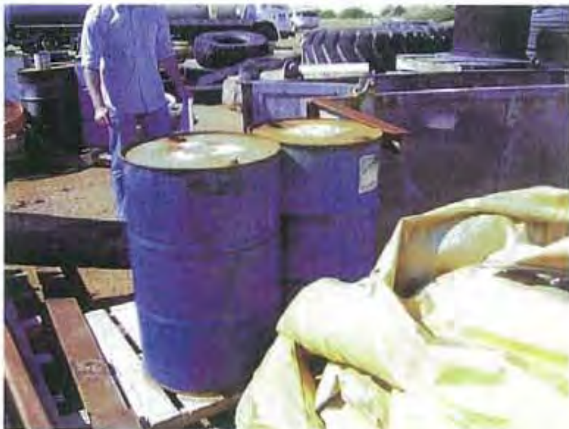
Photo 51: Two 55-gallon drums of used oil were observed stored without secondary containment on the shore side staging area beside the Lil' Perris dry dock.
