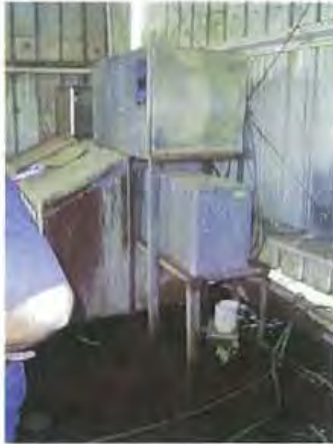
Photo 38: A closer photograph of the runoff from the cement mixing going under the wall of the work barge. Further, the Facility representative stated that condensate from the ice maker discharges under the wall and over the side of the work barge as well.
