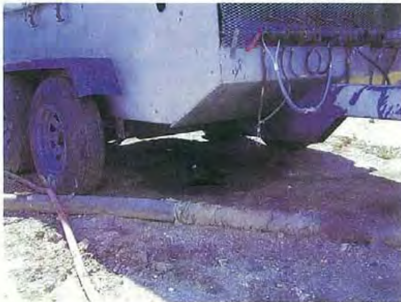
Photo 53: A mixture of oil and condensate dripping from the above pictured air compressor.
