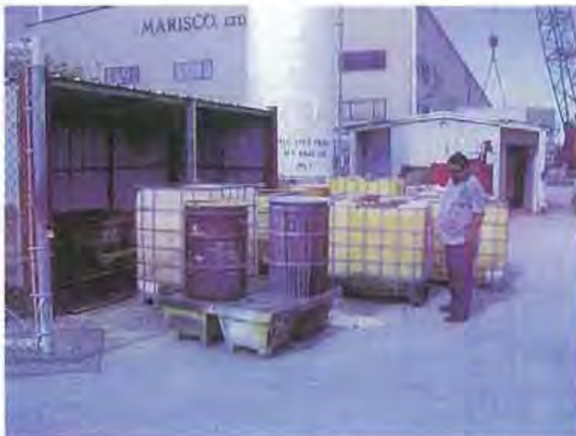
Photo 34: Hazardous waste storage area located adjacent to the main yard entrance of the Facility. Additional drums of paint related waste is shown above, outside the hazardous waste containment area. The white tote has been filled with diesel fuel and is inappropriately labeled as flocculent. Approximately 11 totes were observed in the area, outside any containment area, with residual liquid.
