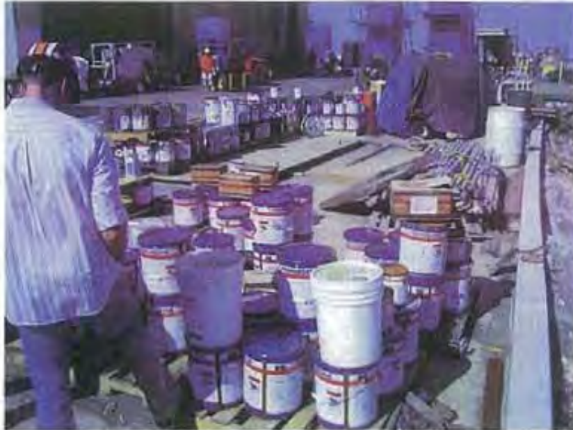
Photo 14: Large quantity of buckets of paint and paint thinner were observed in the yard, uncovered and without secondary containment. The Facility representative stated that this was a temporary measure while they cleaned out their paint storage lockers.
