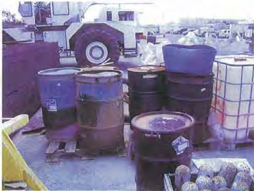
Photo 29: Three of the 55-gallon drums pictured (and labeled) above appeared to contain petroleum products, including motor oil and diesel fuel. These drums are not in a contained area, do not have secondary containment, and are exposed to potential rain fall.
