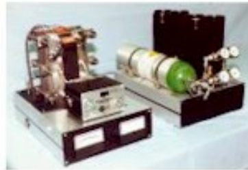
Demonstrator Power Plant - 2 kW
