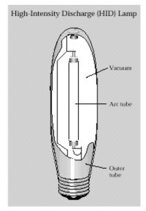
In a high-intensity discharge lamp, electricity arcs between two electrodes, creating an intensely bright light. Mercury, sodium, or metal halide gases act as the conductor.
