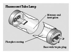
In fluorescent tubes, a very small amount of mercury mixes with inert gases to conduct the electrical current. This allows the phosphor coating on the glass tube to emit light.
