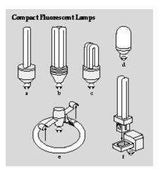
Compact fluorescent lamps come in a variety of sizes and shapes including (a) twin-tube integral (b and c) tripletube integral, (d) integral model with casing that reduces glare, (e) modular circline and ballast, and (f) modular quad-tube and ballast. They can be installed in regular incandescent fixtures, and they consume less than one-third as much electricity as incandescent lamps do.
