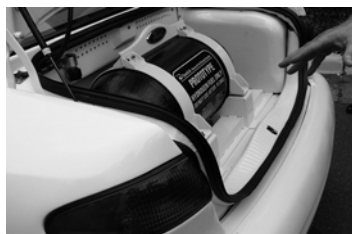
compressed hydrogen gas tank
