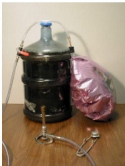
Completed biogas generator.
