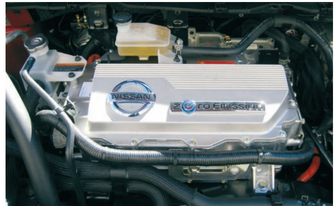
Under the hood of a Nissan Leaf. An EV contains no ICE. Instead, the battery supplies electricity to the electric motor. Photo from Margaret Smith, DOE, NREL 18218
