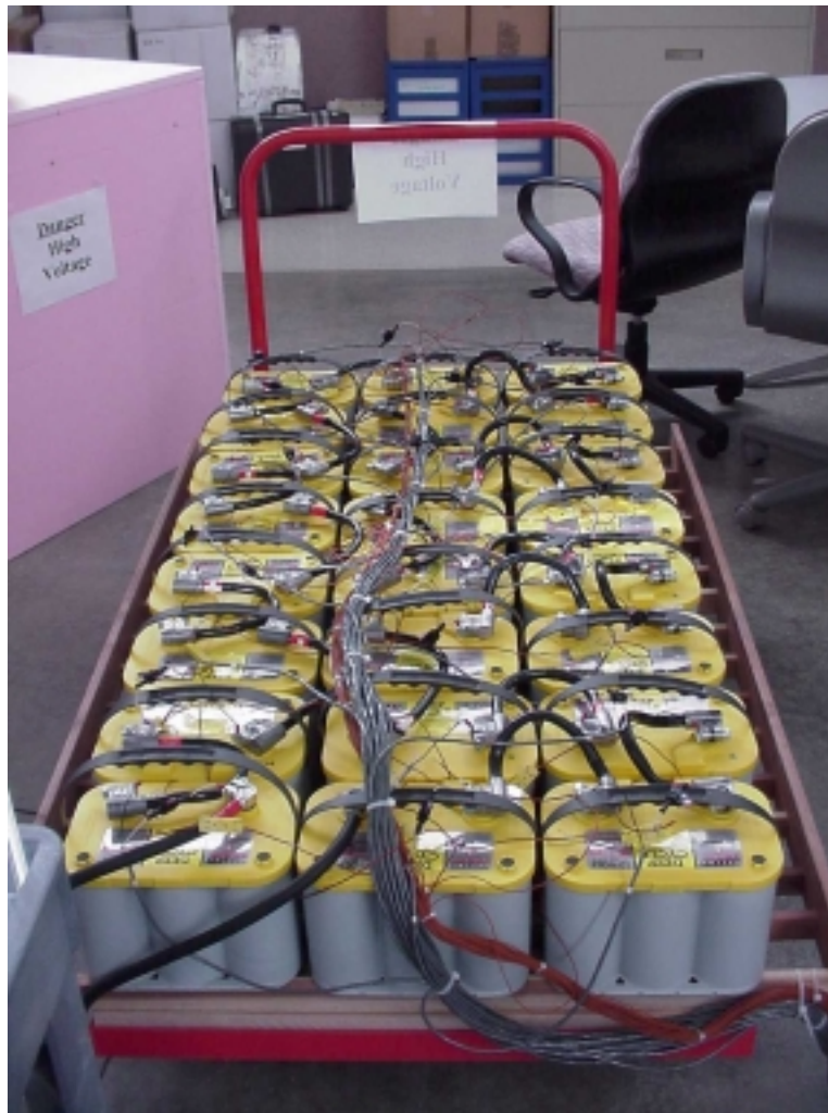
Figure 8 Optima Battery Pack Used to Test Cycle Life
