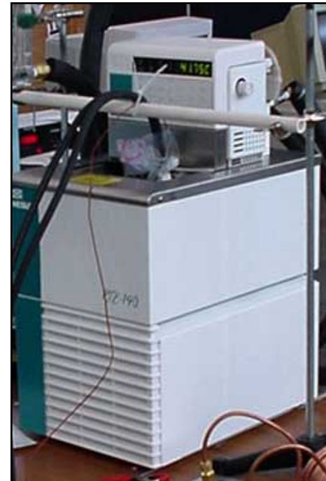
Temperature Testing in NESLAB Liquid Bath
