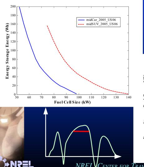
Battery provides peak shaving capability during the US06 drive cycle
