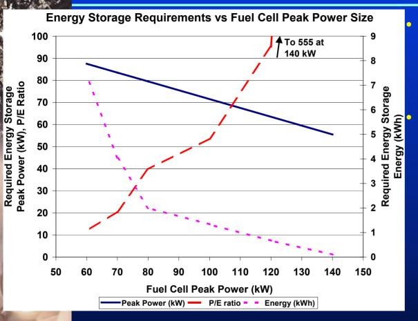
Energy storage power (P), energy (E), and P/E ratio are compiled for many fuel cell sizes.
