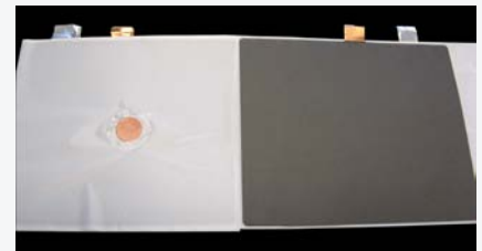
NREL's internal short placed within a pouch cell. Photo by Dirk Long, NREL
