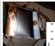
BISCD implantation in 18650 cell. Photo Credit: Mark Shoemith, E-One Moli
