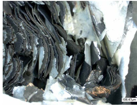
Fracture of multiple layers during a crash/impact test
