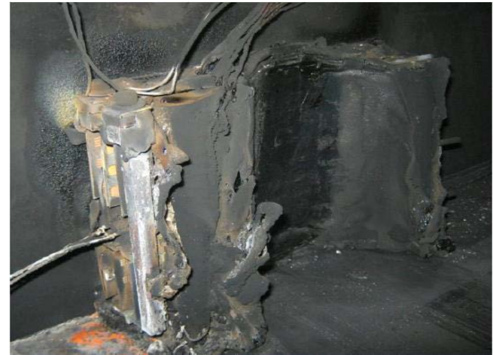
Slow crush of a battery module
