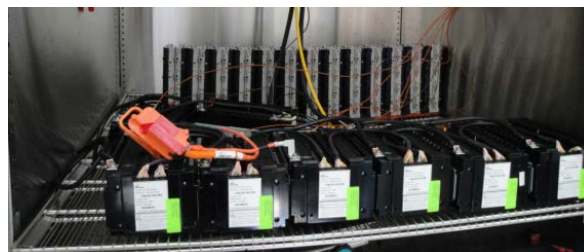
Figure 3. JSR LIC modules in an environmental chamber during bench testing, with the production 2012 Fusion Hybrid NiMH modules in the background (Photo credit: John Ireland, NREL).
