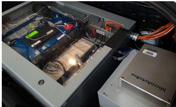
Figure 12. Installed Maxwell EDLC seven-module configuration (Photo credit: Jon Cosgrove, NREL).
