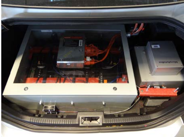
Figure 4. Fully integrated conversion system mounted in the trunk of the Fusion Hybrid test platform (Photo credit: Jon Cosgrove, NREL).
