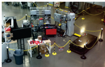
Grid Simulator: Elgar SW15750 Grid Simulator – 15.75 kVA Load Bank: Simplex PowerStar 100 Resistive Load Bank – 100 kW PV Simulator: TerraSAS ETS1000X PV Simulator – (2) Parallel 10 kW Modules Real-Time Interface: Opal-RT eMegaSim Wanda 4U 16-core Real-time Simulator
