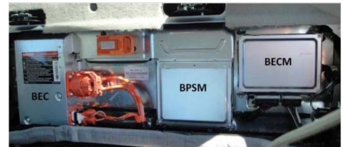
Fusion test platform and traction battery with Bussed Electrical Center (BEC), Battery Pack Sensor Module (BPSM), and Battery Energy Control Module (BECM)
