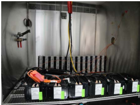
Figure III.C.2.4-4: JSR LIC modules in an environmental chamber during bench testing, with the production 2012 Fusion Hybrid NiMH modules in the background (Photo credit: John Ireland, NREL)
