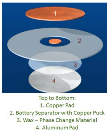
Figure III.D.6-1: ISC schematic—not to scale
