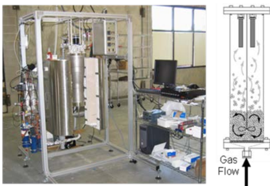
Figure IV.D.4-1: Fluidized bed reactor to coat powders with ALD cycles; the existing reactor at ALD Nanosolutions can process up to 8L of powder per batch
