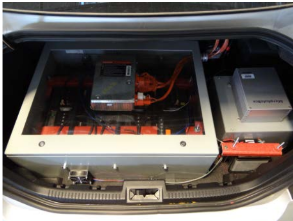
Figure III.C.2.4-7: Fully-integrated conversion system mounted in trunk of Fusion Hybrid test platform (Photo credit: Jon Cosgrove, NREL)
