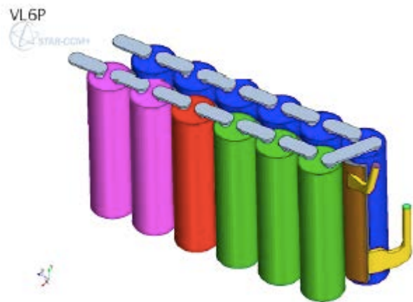
Figure III.E.4-6: STAR-CCM+ model of cell components
