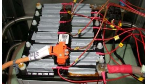
Figure III.E.3-9: Module validation test setup for full-field simulation against test data for high-frequency pulse charge-discharge
