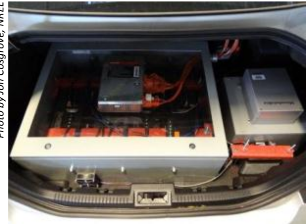
Simulink state estimation model currently deployed on the MABx for control, and photo of LEESS installation in the trunk space showing the JSR LICs and MABx
