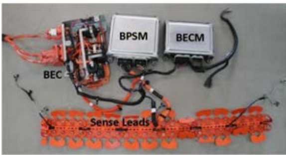
Figure III.C.2.4-2: Replacement interface components for use with the alternate LEESS; Photo credit: Ahmad Pesaran, NREL
