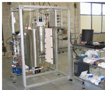
Figure IV.B.2.5-1: Fluidized bed reactor to coat powders with ALD cycles: the existing reactor at ALD Nanosolutions can process up to 8L of powder per batch; Photo credit: Shriram Santhanagopalan, NREL
