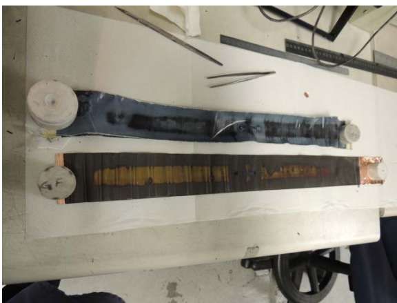
E-One Moli 18650 cathode and anode assemblies unrolled after ISC activation; Photo credit: Dirk Long, NREL
