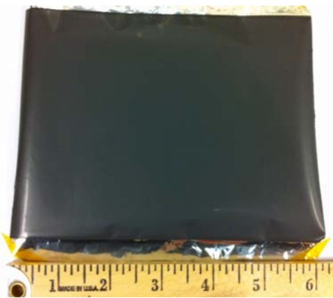
Figure IV.B.2.4-7: A 6-in by 6-in foil of Toda HE5050 following coating with 5 cycles of ALD alumina; Photo credit: Rob Tenent, NREL
