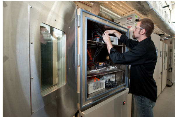
Life cycle testing of batteries for secondary-use applications; Photo credit: Dennis Schroeder, NREL
