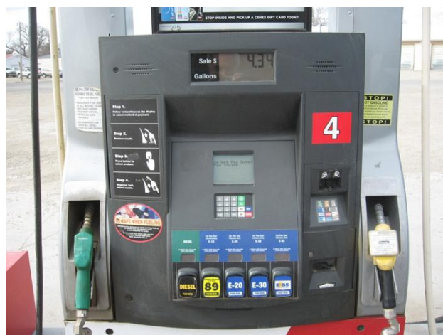
FIGURE 3. Example of Station Offering Higher Ethanol Blends from the same Hose as E10
