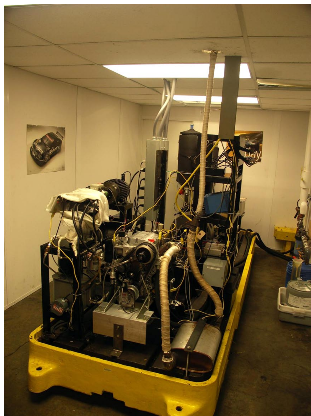
FIGURE 4. A Kohler 16-hp twin-cylinder diesel engine on a dynamometer test bed.
