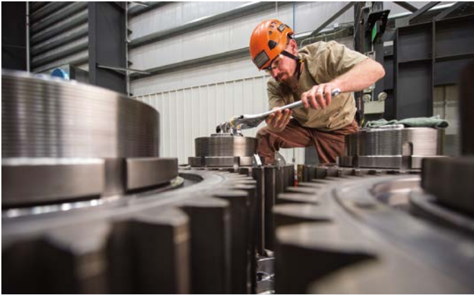
NREL technician working on a lubrication manifold of a next-generation drive train for a wind turbine gearbox. Photo by Dennis Schroeder, NREL 32786
