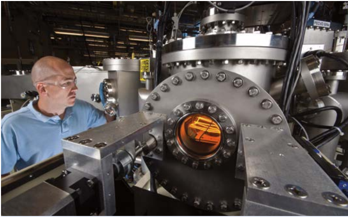
An engineer operating the silicon cluster tool in the Science and Technology Facility. The tool is used to develop techniques to explore and enhance potential industry practices for fabricating silicon solar cells. Photo by Pat Corkery, NREL 16555
