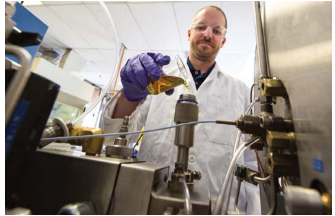
NREL researcher uses a small quantity of biofuel to evaluate the combustion kinetics in an Ignition Quality Tester at an NREL Denver West laboratory. Photo by Dennis Schroeder, NREL 32870
