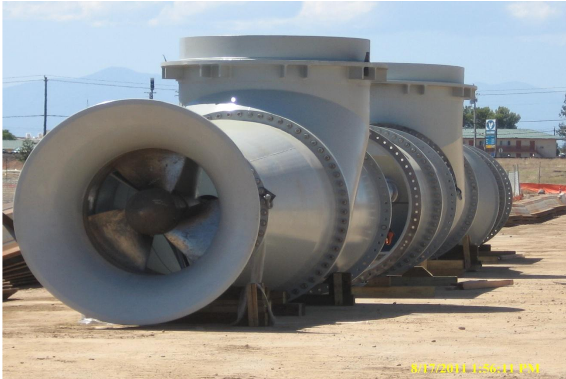
84-inch pumps #2 and #3 delivered to Balfour Beatty Infrastructure and set in storage.
