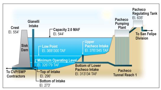
Figure 1-4. Reservoir Intake and Outlet Facilities
