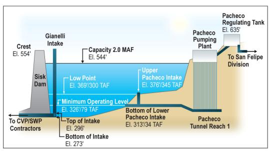
Figure ES-2. Reservoir Intake and Outlet Facilities
