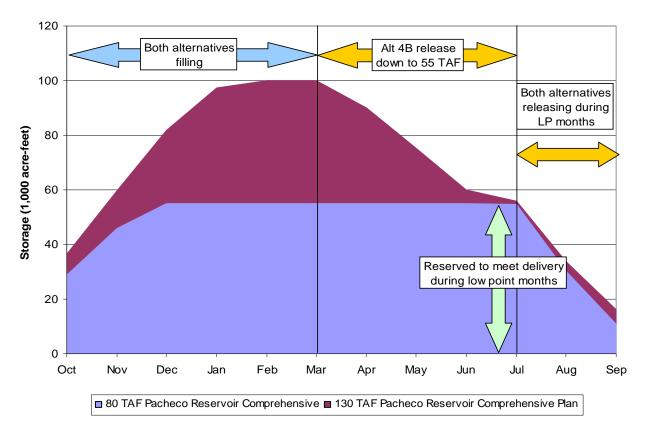
Figure A-25. Typical Pacheco Reservoir Operations
