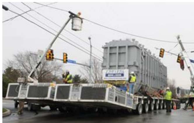
Figure 4. Transport of Large Power Transformers
