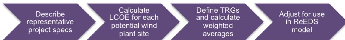
Figure H-9. Land-based wind plant cost and performance techno-economic parameter calculation process
