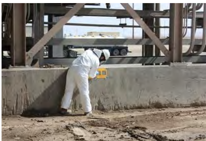
Figure 1 Canon EOS Rebel XSi, Photo #20; PCB wipe sampling at location CH-1935-WP-04, facing east-southeast
