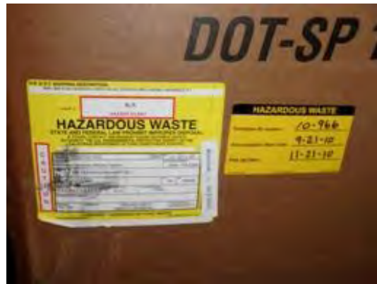
Olympus Stylus 8000, Photo #29; DSHA Staging Area. View of a cardboard container of crushed containers with an incorrect accumulation start date (pickup date) of 11/21/10.
