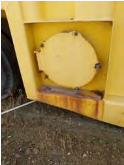
Olympus Stylus 8000, Photo #56; View of the leachate collection frac tank at WMU 34, facing east. Note the stains around the valve area and on the ground.
