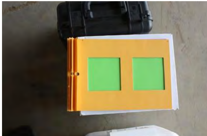
Canon EOS Rebel XSi, Photo #6; View of the PCB wipe templates (two, 10cm x 10cm squares cut in each template).
