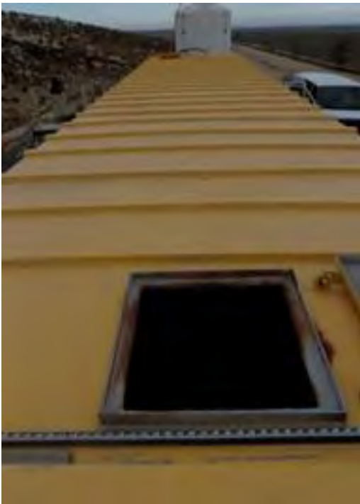
Olympus Stylus 8000, Photo #97; View of the leachate collection frac tank (Tank 80) at WMU 35, Cell #1. Note the top of the container is open.
