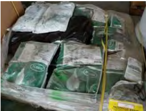
Olympus Stylus 8000, Photo #40; Another view of the waste fertilizer bags (California hazardous waste) shown in Photo 36. Minor rips are present in the bags and the top of pallet is not covered or wrapped. Photo to the left.
