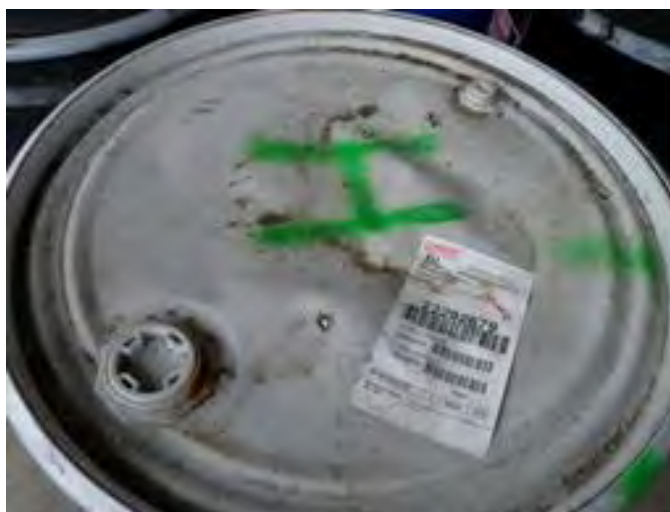
Olympus Stylus 8000, Photo # 16; View of a 55-gallon container in DSHA Area 4, holding waste lead paint chips, dated 9/21/10. The lid is dented, but no evidence of leaks or releases.
