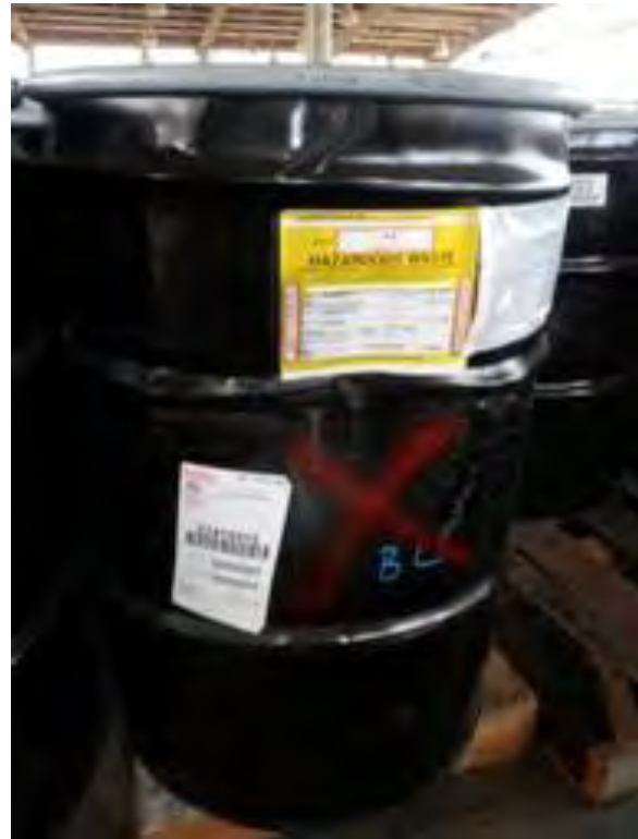
Olympus Stylus 8000, Photo #27; DSHA Staging Area. View of a dented container of a California hazardous waste. No visible leaks or releases.
