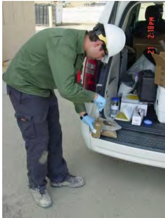
Sony DSC-S75, Photo #24; PCB soil sampling. Homogenization of soil and filling the sample container, facing north.
