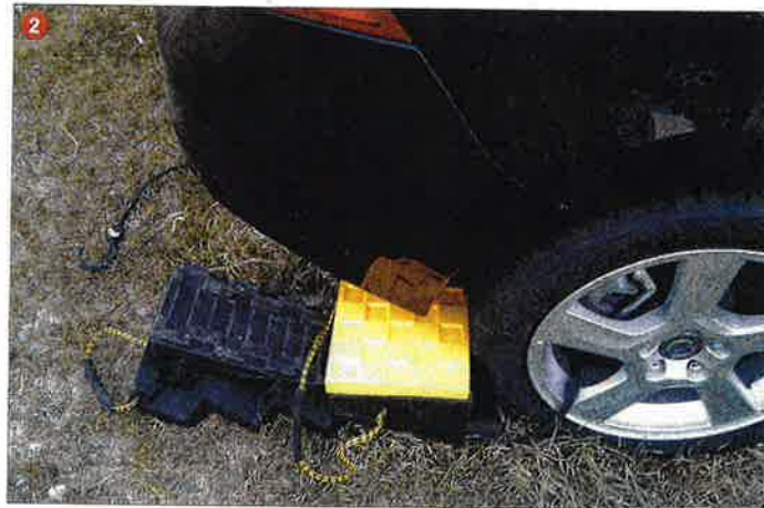
(2) The user positions the Cog Step as needed, with the cog wedge in close proximity to where it is needed to effect stabilization. As rescuers unweight the side of the vehicle, as they would place a standard step chock, they introduce the Cog Step in much the same way. (Photo by author.)
