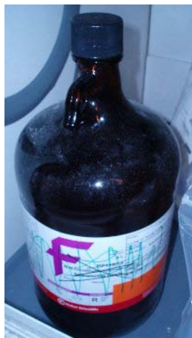
Photo 8: unlabeled hazardous waste bottle
