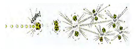
Nuclear fission—each "fission" of a <sup>235</sup>U atom by a neutron results in release of radiation (heat, light, gamma and x rays), more neutrons, and other particles.
