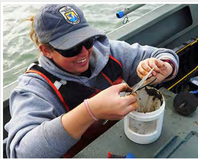
Fisheries technician Jessica Loughner scrapes organisms and organic matter off of a Hester-Dendy trap that was set in Maumee Bay, Lake Erie. Credit: Andrew Briggs, USFWS
