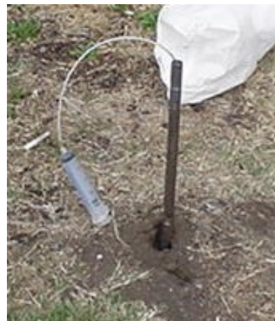
Figure D-1. Hollow rod used to collect soil gas.
