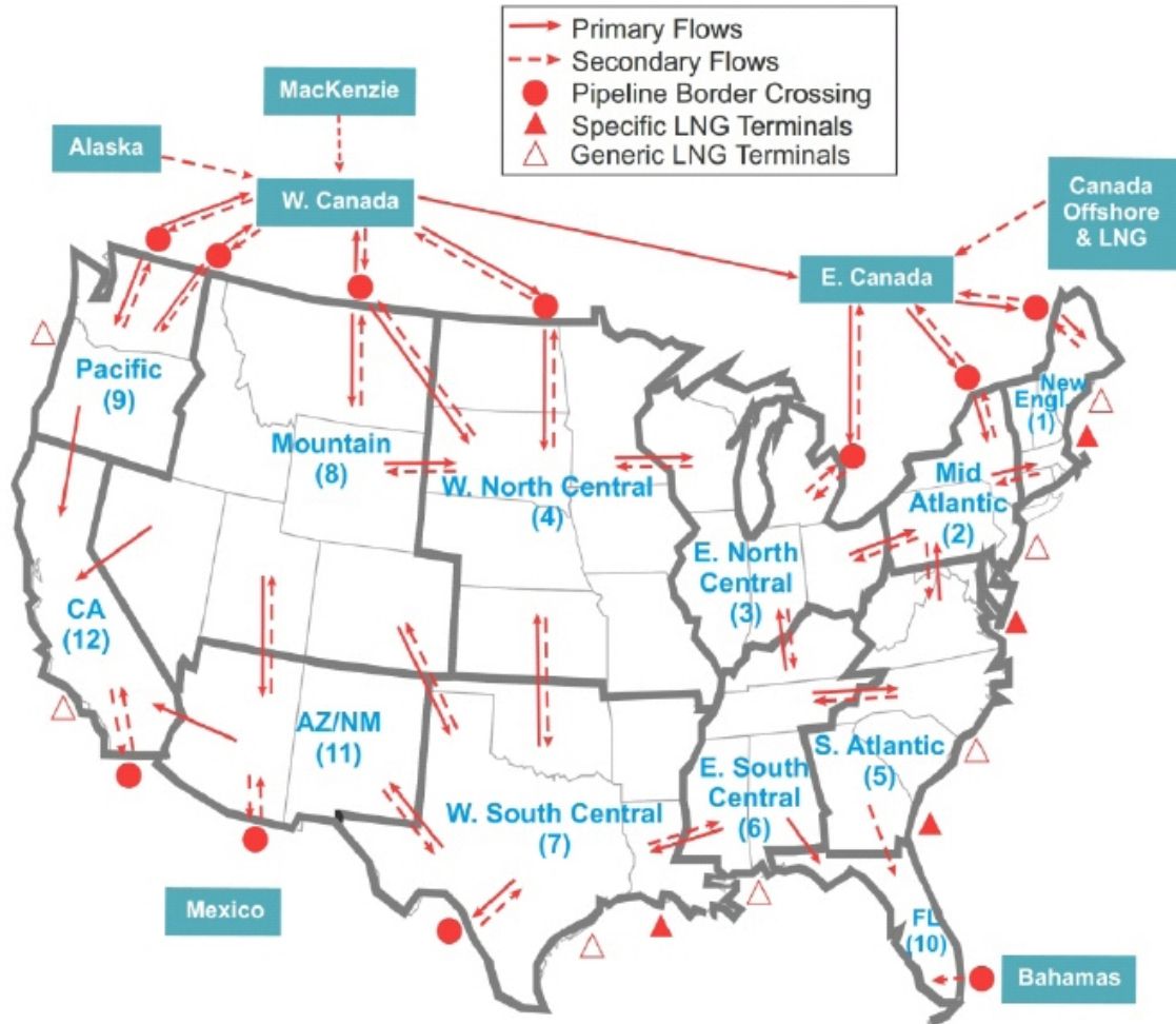
Figure 15. Natural Gas Transmission and Distribution Module Network
