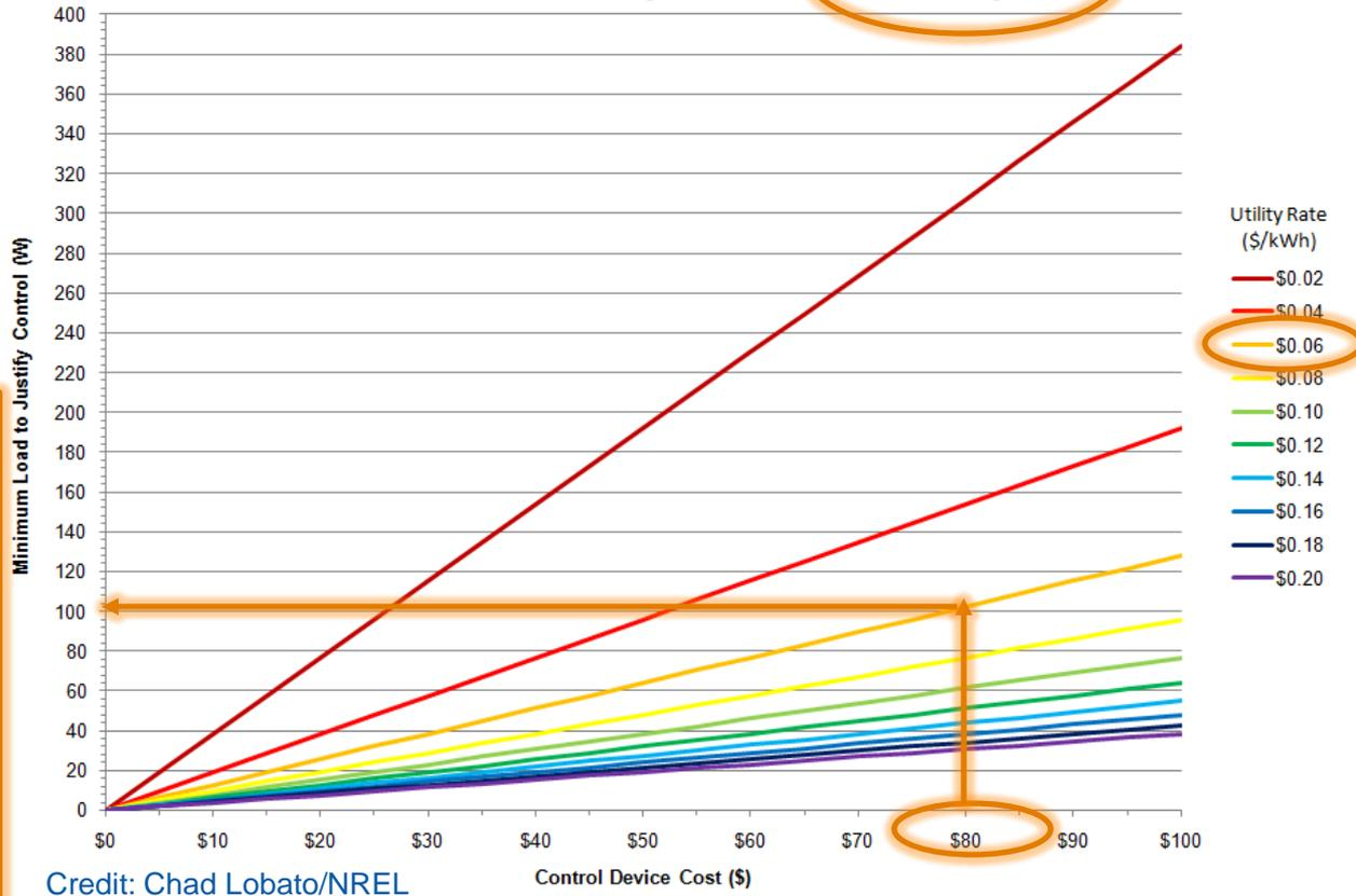
Based on an example office equipment schedule, selected payback, utility rate, and device cost, any load greater than 100 W is cost effective to control.
