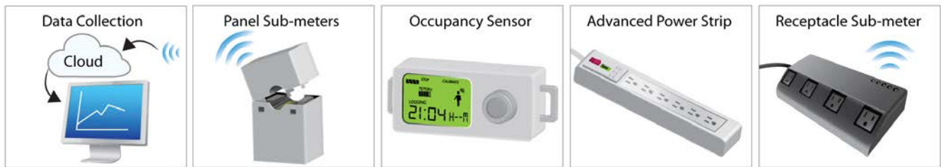
Figure ES-2. Close-up views of sub-metering, control, and occupancy monitoring components that were installed and demonstrated in Building A4. Illustration by Marjorie Schott, NREL
