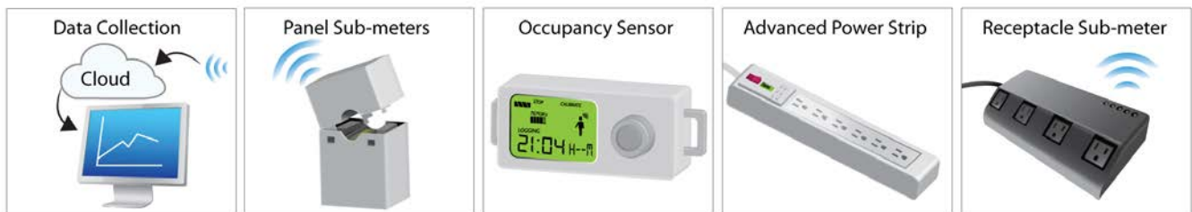
Figure 2. Close-up views of submetering, control, and occupancy monitoring components that were installed and demonstrated in building A4. Illustration by Marjorie Schott, NREL
