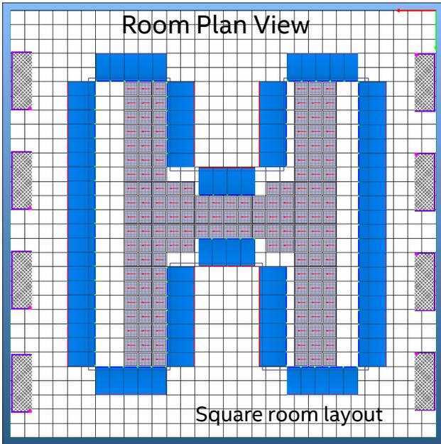
This layout provides 40% more rack bays than racks placed as a square perimeter
