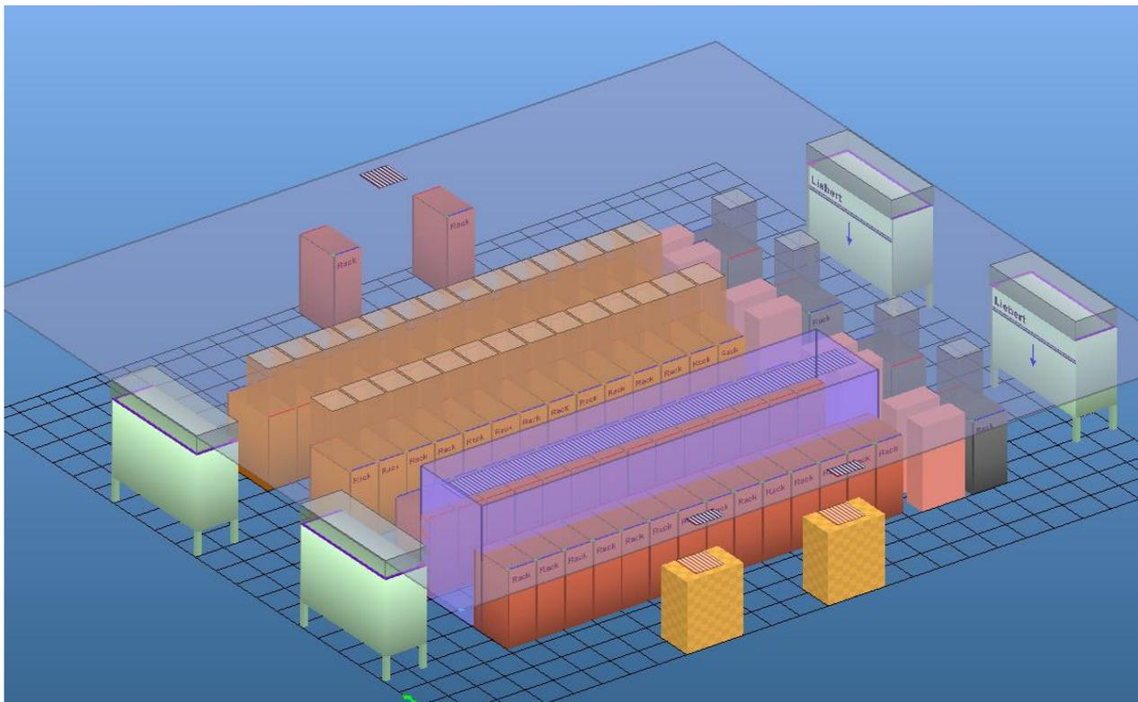
Raising the air handlers above the raised metal floor allows a room with poor underfloor distribution or capacity to increase the effective cooling density.
