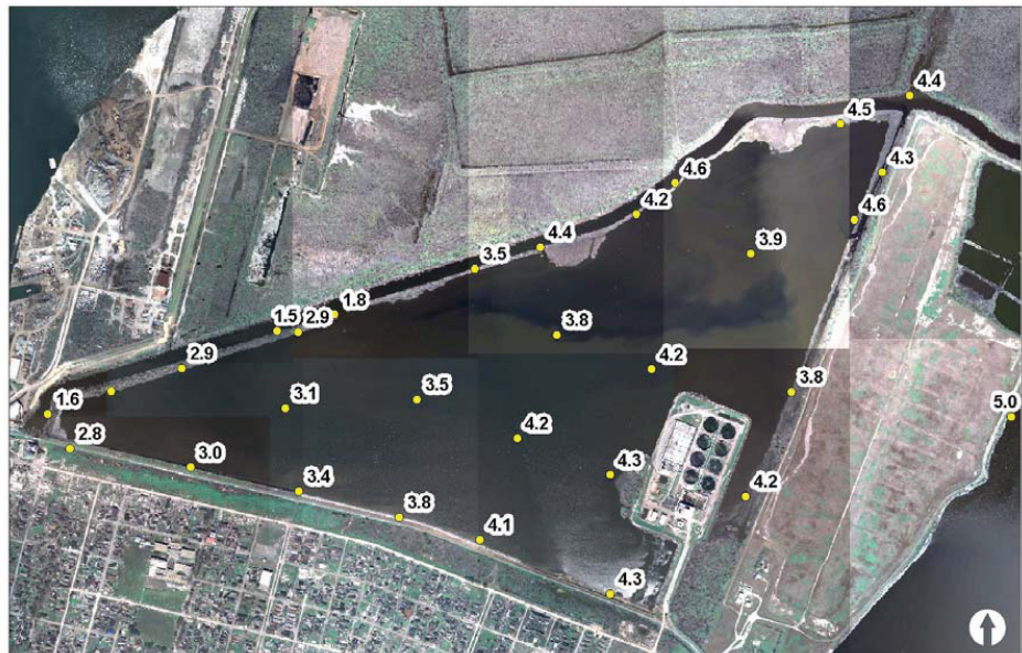
Figure 4-14. Surface-water salinity (in ppt) in the Bayou Bienvenue Wetland Triangle, June 2007.
