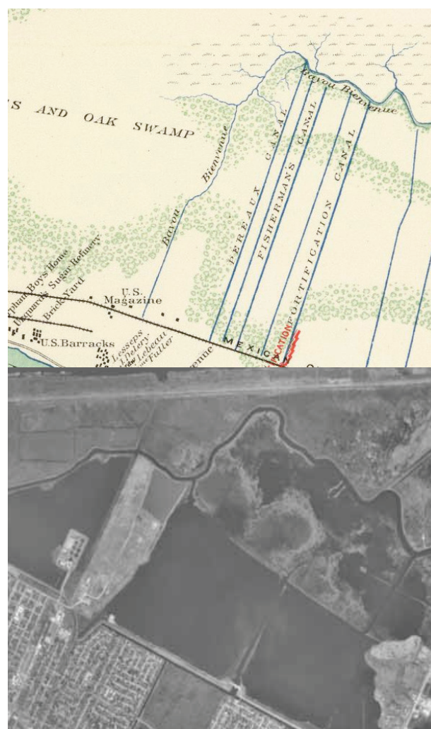
Figure 1-5. Comparison of the main outfall canal from Pumping Station no. 5 prior to its construction with modern Bayou Bienvenue. The natural drainage pattern can be discerned. Map: ( http://www.davidrumsey.com/detail?id=1-1-26919-1100218&name=Approaches+to+New+Orleans ). Aerial photo: (TerraServer-USA, Microsoft Corp, USGS).
