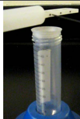
Position of rod over conical tube during carrier deposition (the rod must not touch the splashguard insert)
