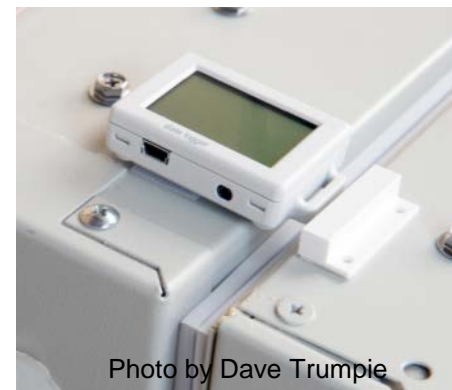
Door Openings: Magnetic State Logger
