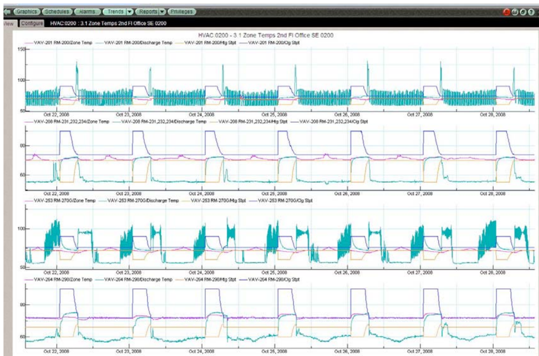
Figure 3: Diagnostic trends of VAV zone temperatures
