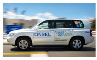
The Toyota FCHV-adv design is representative of the fuel cell vehicles that many automakers are expecting to release commercially in the 2015–2017 timeframe. *Photo by Dennis Schroeder, NREL 25255*
